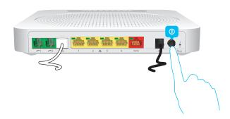
4 The (1) LED turns on. Wait at least two minutes to allow your TG789vac v2 to complete the startup phase.
